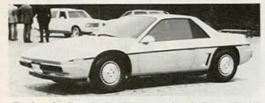
Two days after the studio photo (above) was taken, the Pontiac II model was presented to management for approval. Even though this model looks like the final Fiero, the front humper, side air intakes, and rear taillamps are still not yet production-ready. At the time of the presentation, the P was no longer called the Sprint; the model carries P5000 identification.
